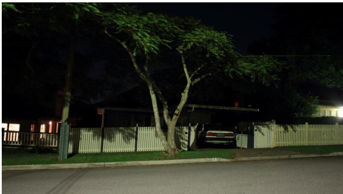
Even though Emma Street is wide this luminaire still causes forward light trespass.
