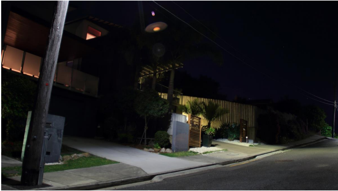
The sharp cut-off of the primary beam below the luminaire creates areas of deep shadow for pedestrians and highly variable footpath illumination that progress from intensely bright to tolerably bright again and again along the street.
