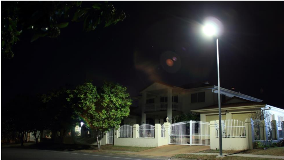
Malbon street – west. Excessive rear light trespass.
