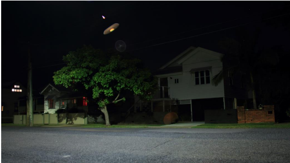
Forward light trespass and secondary glare zone trespass on to private property.
