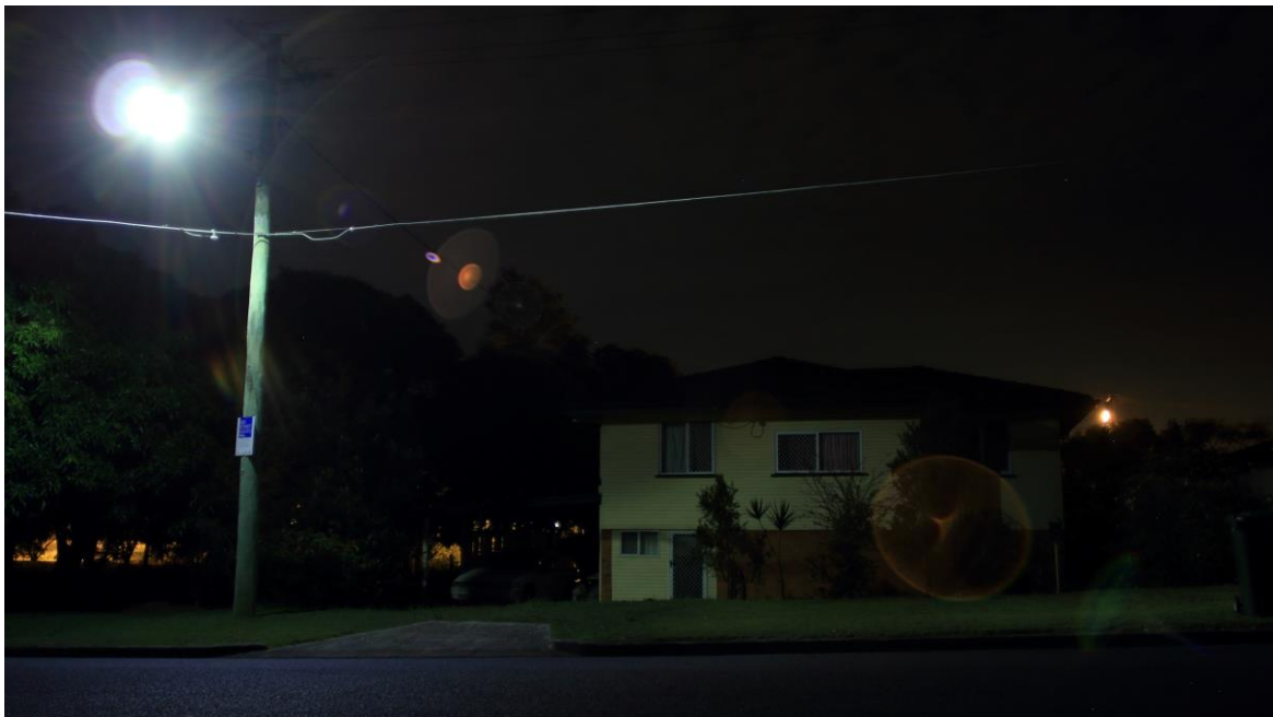
Excessive rear light trespass on to private property.
