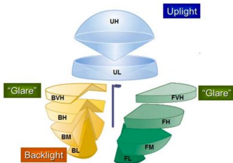
Figure 9 BUG scale of luminaires. (Miller et al., 2013, IDA/IES, 2011)
