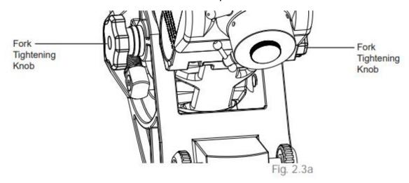
Adjust the elevation with the Latitude Jackscrew. End the elevation adjustment with an upwards movement of the Latitude Jackscrew. Then retighten the Fork Tightening Knobs.
